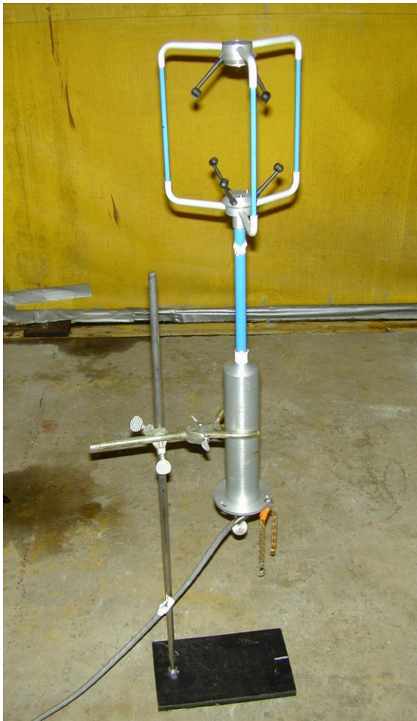
Figure 5: The Gill 3-Axis Sonic Anemometer on a laboratory stand.
